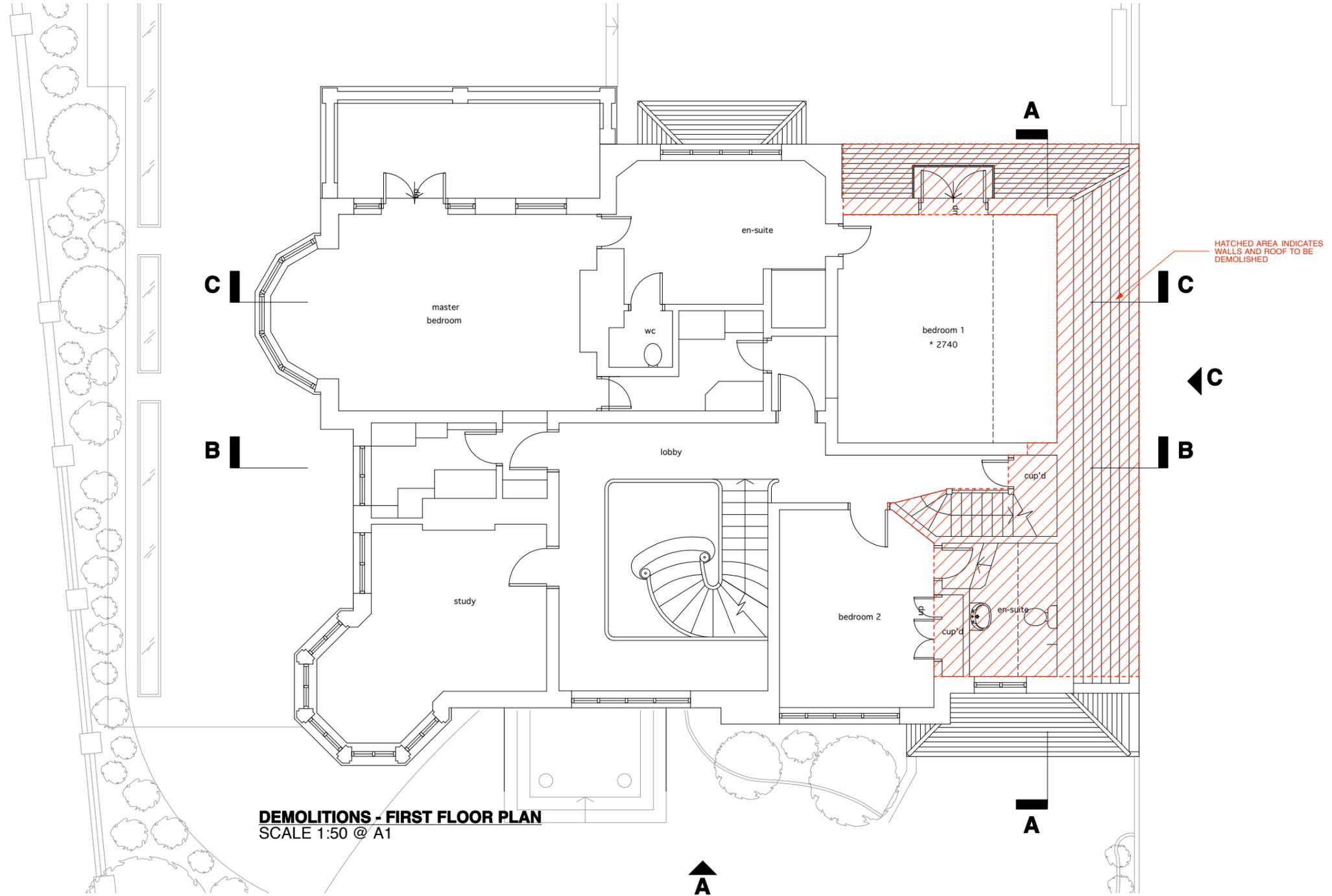
HATCHED AREA INDICATES WALLS AND ROOF TO BE DEMOLISHED
