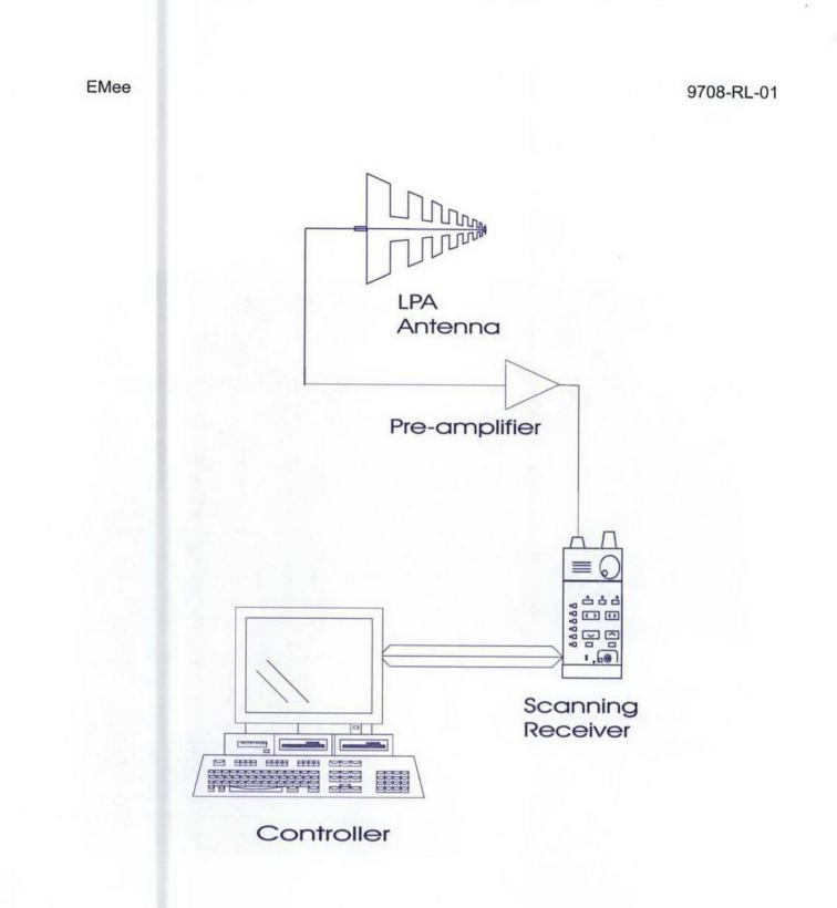
Fig.A.2 : Test Schematic - Signal Strength (450MHz - 650MHz)
