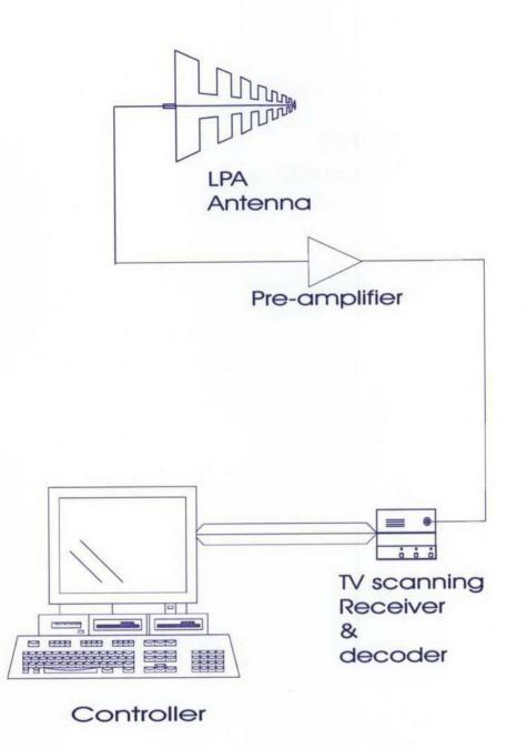
Fig.A.3 : Test Schematic - Reception Quality
