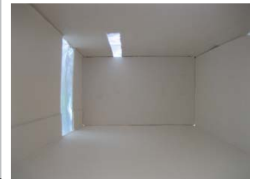
Model to show light condition from new roof light
