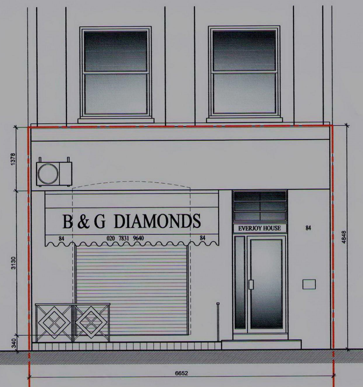
Front Elevation - As Existing
