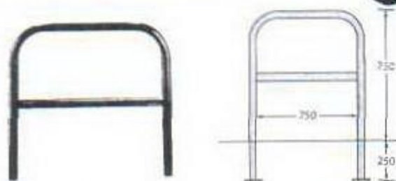
SHEFFIELD CYCLE STAND WITH TAPPING BAR
