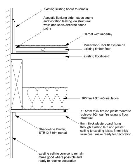
**Detail Section** Scale 1:5 ■ Ceiling/Floor Detail 2nd & 3rd Floor
