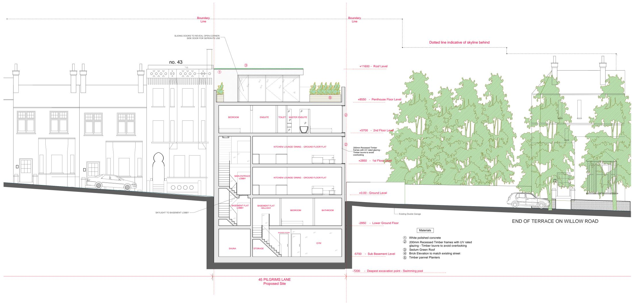
SCALE: 1:200 @A3 1:100 @ A2 NOTES: Revisions Section BB @ A2 Report all errors and discrepancies promptly to architects before proceeding with the works.
