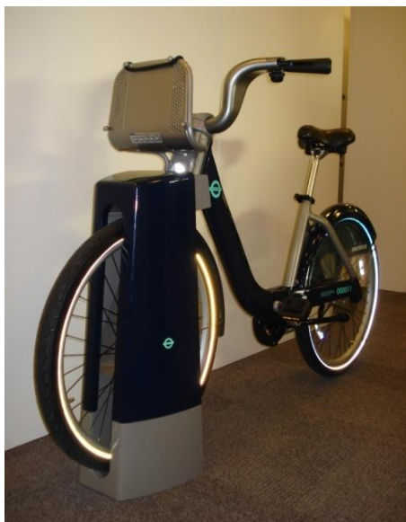
Figure 2: Docking point with docked bicycle
