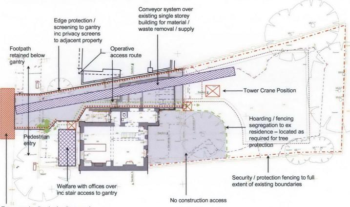
Temporary loading / unloading area / used for Mobile cranes as required. Suspension of parking bays for deliveries to be agreed with LA / highways
