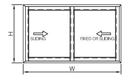
Width Max 3000 mm Height Max 1800 mm
