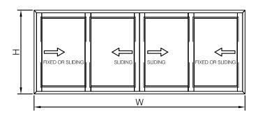
Width Max 6000 mm Height Max 1800 mm
