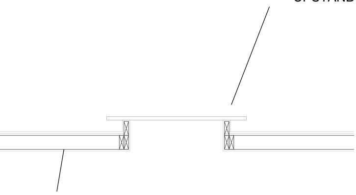
EXISTING TIMBER FLAT ROOF CONSTRUCTION CONTINUED LIKE FOR LIKE ON TO EXTENSION ROOF
