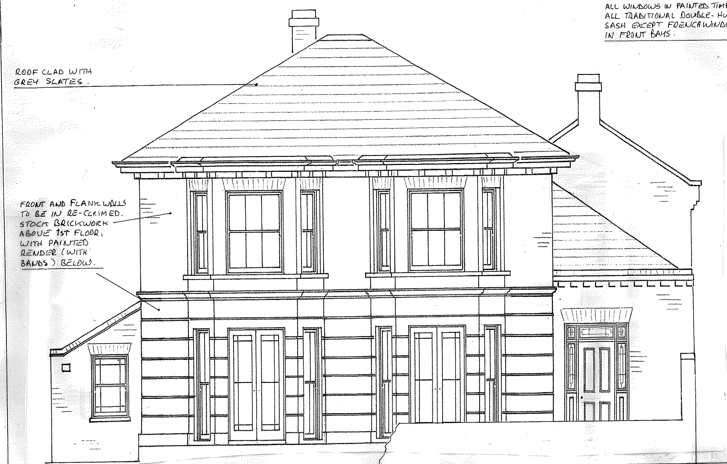
SOUTH FRONT ELEVATION (HURRAY ST. SIDE)
