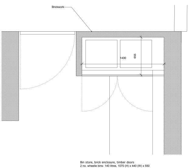
0m Bin store, brick enclosure, timber doors 2 no. wheelie bins- 140 litres, 1070 (H) x 440 (W) x 550 (D) 1:20 / A3
