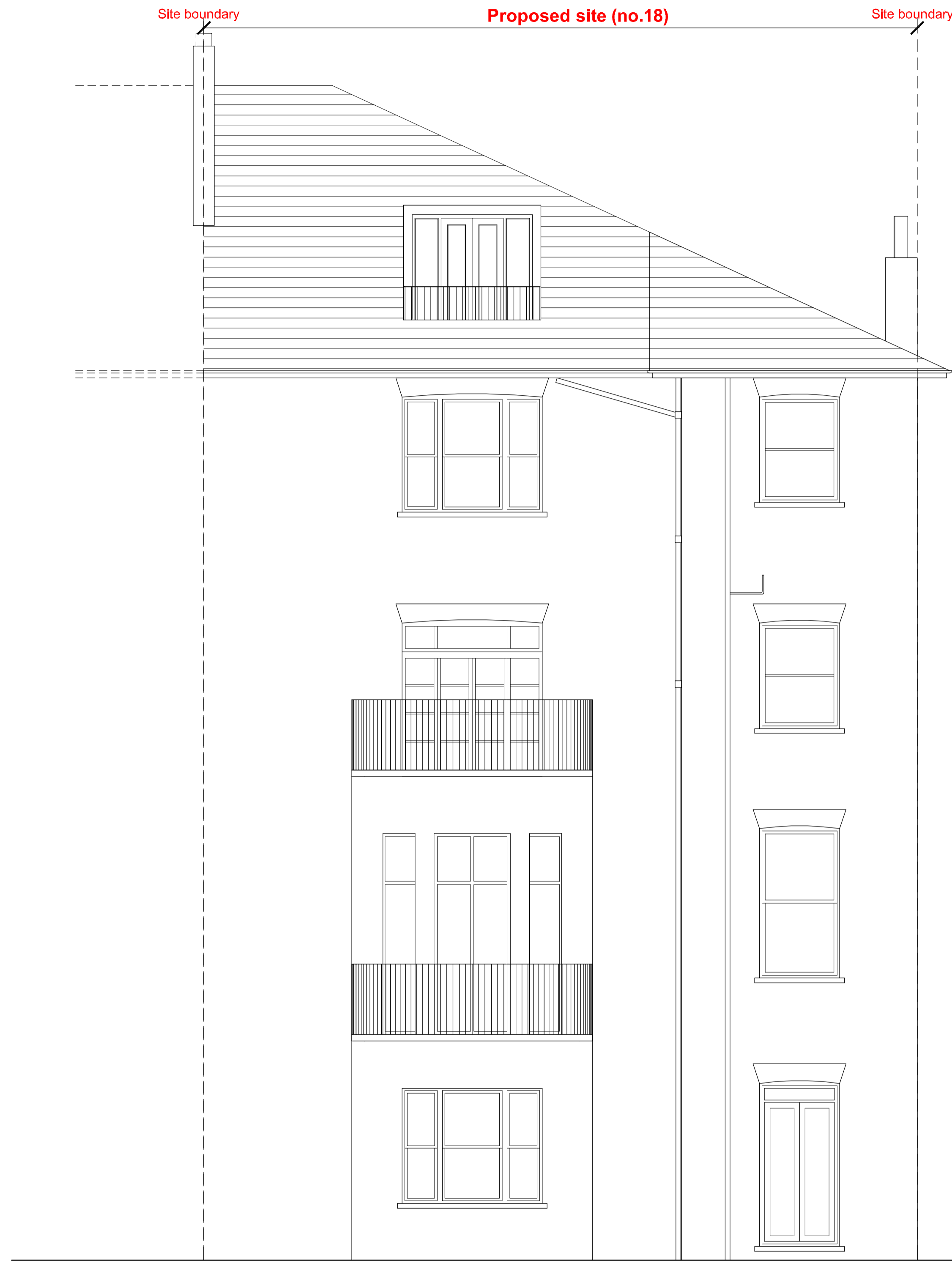
REAR (NORTH) ELEVATION
