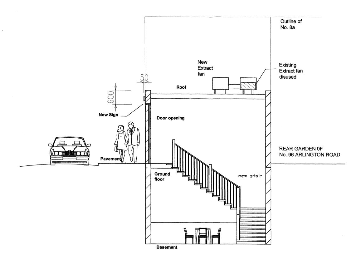
AS CONSTRUCTED CROSS SECTION AA AT STAIRS
