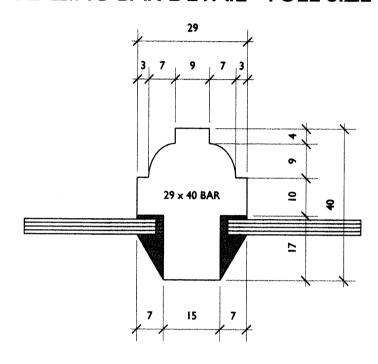
PROPOSED NEW GLAZING BAR DETAIL TO EXACTLY MATCH ORIGINAL ADJACENT SLIDING SASHES.
