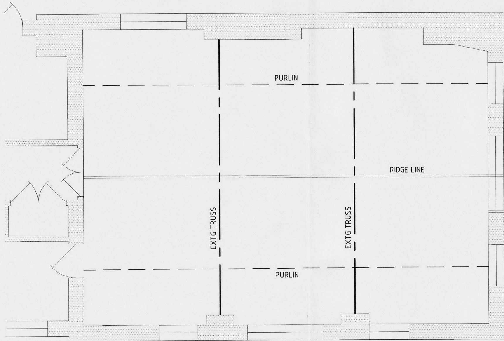
EXISTING STRUCTURAL PLAN
