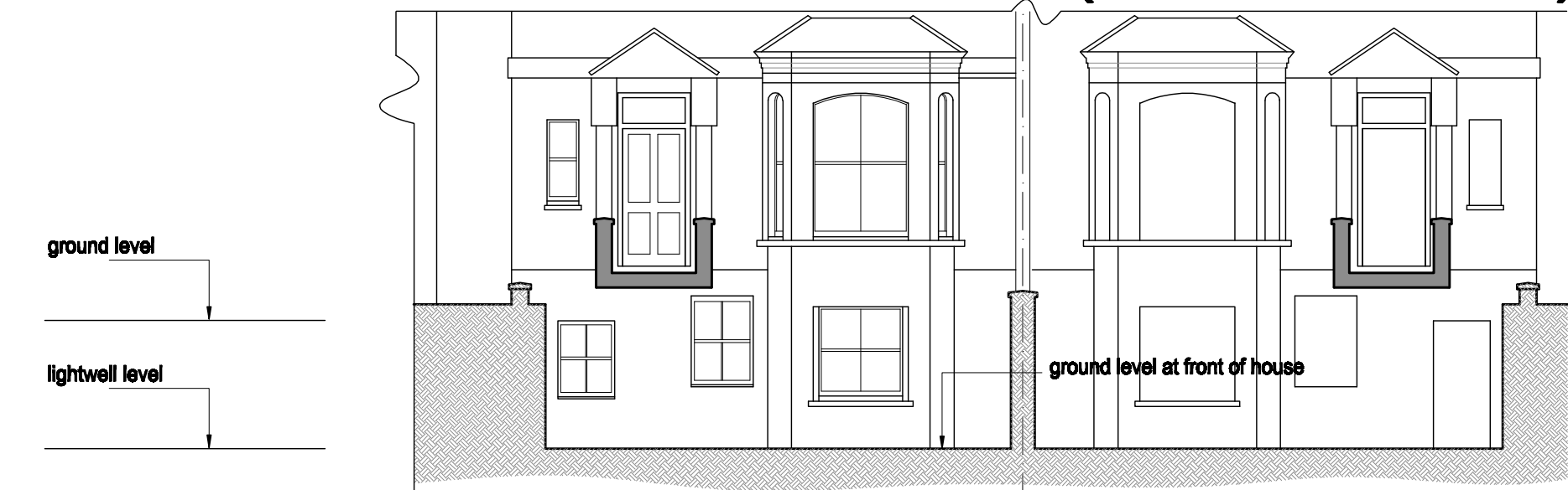
Lightwell Elevation (section D - D) as existing
