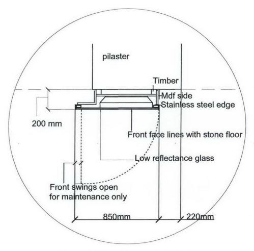
Plan section CC of one of the two monitors, detail east side, as proposed
