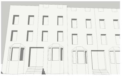
3D views showing that the proposed mansard extension is not visible from the street below, and is largely hidden by the existing parapet on the front elevation
