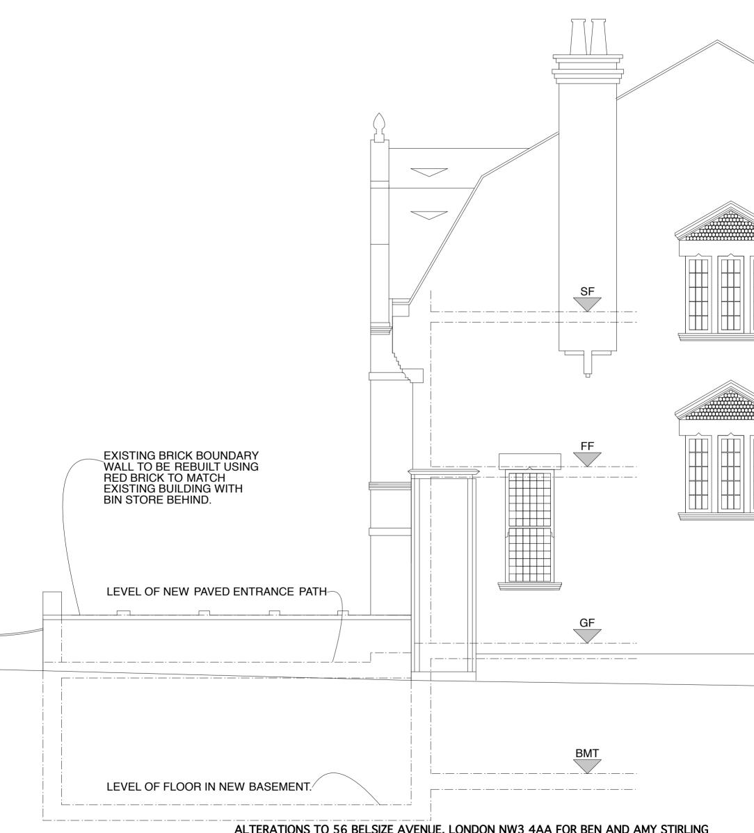
ALTERATIONS TO 56 BELSIZE AVENUE, LONDON NW3 4AA FOR BEN AND AMY STIRLING SIDE ELEVATION AS PROPOSED scale 1:50@A3 date 14 06 10
