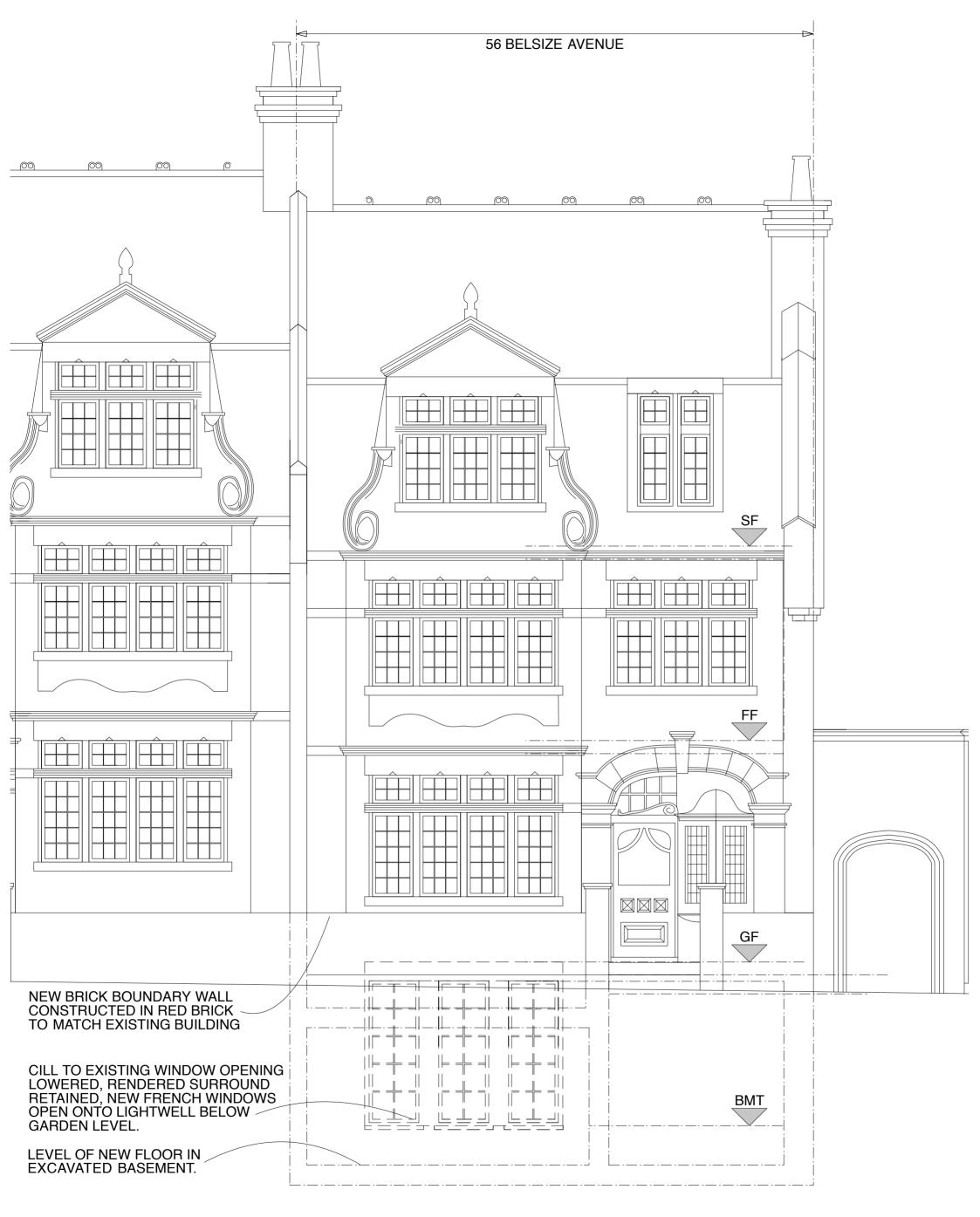
ALTERATIONS TO 56 BELSIZE AVENUE, LONDON NW3 4AA FOR BEN AND AMY STIRLING FRONT ELEVATION AS PROPOSED SHOWING GARDEN WALL.
