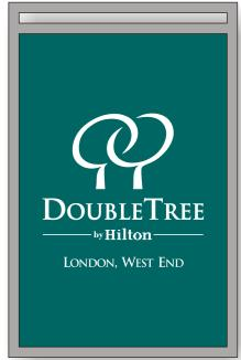
Sign 2 - 2No. double sided projecting signs internally illuminated. 100mm x 1500mm.
