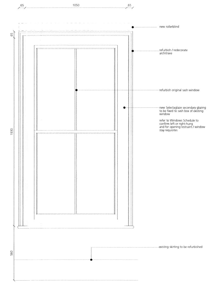
1 WG.04 Proposed Elevation 1:10 @ A1
