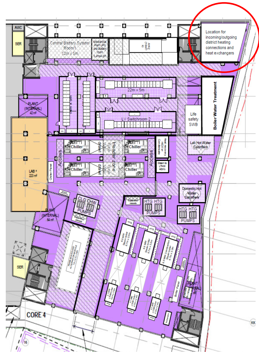
Figure 7-3. UKCMRI Level -1 Plant Layout illustrating space (red circle) available for connection to an external heat network
