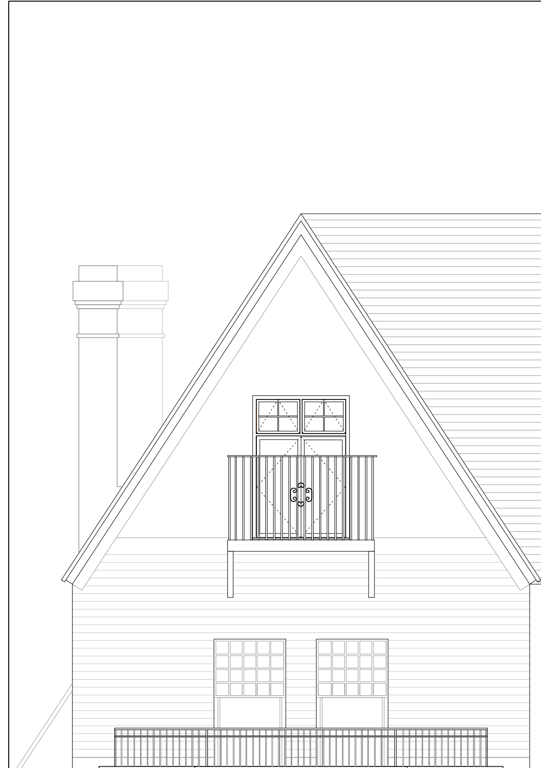
PART WEST ELEVATION AS PROPOSED SCALE 1:50
