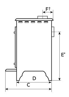
Recommended clearances between stove and other surfaces: top 9" (225mm), sides 6" (150mm), rear must be a minimum of 2" (50mm)
