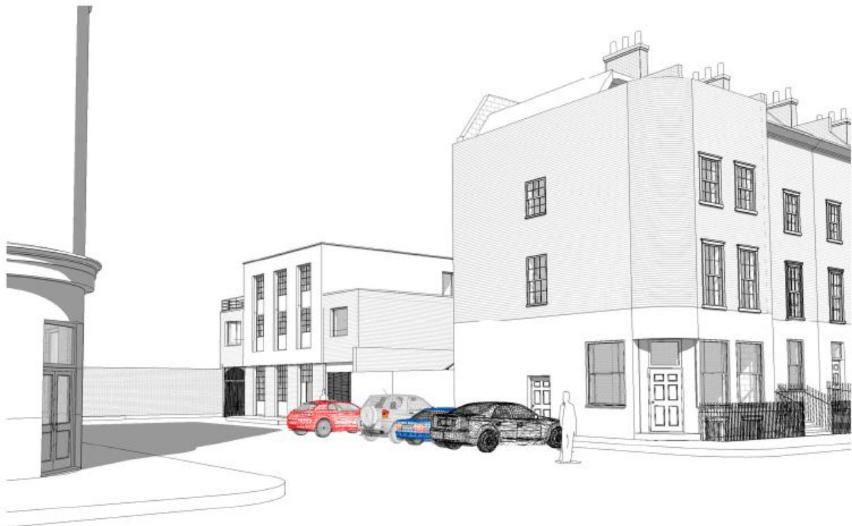
Fig. 1: Visualisation of the proposed office building, echoing the prevailing solid-void ratios and the material palette of properties on Gloucester Avenue in the use of stock brick and light coloured render. (PMA Architects)
