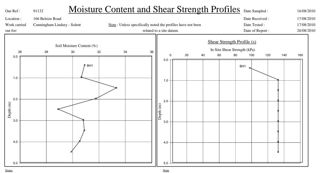
If the Soil Fraction > 0.425mm exceeds 5% the Equivalent Moisture Content of the remainder ( calculated in accordance with BS 1377: Part 2 : 1990, cl.3.2.4 note 1 ) is also plotted and the alternative profile additionally shown as an appropriately coloured broken line.
