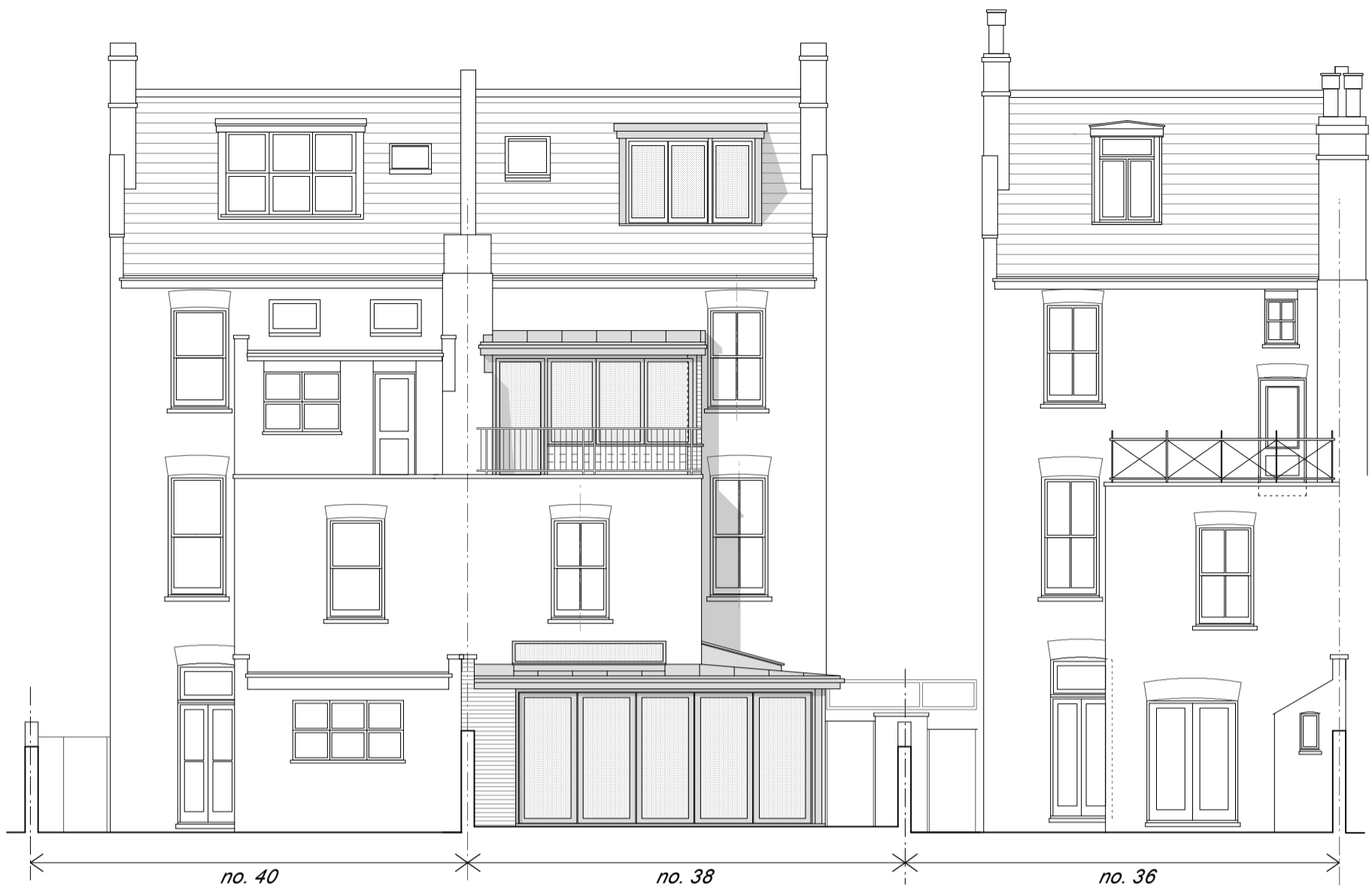
1:100 REAR ELEVATION (NORTH) showing adjoining houses
