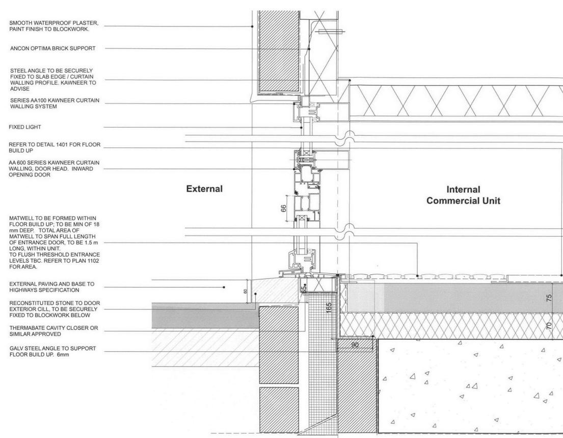
DETAIL 07 Section Retaining Wall/ Door Threshold to Commercial Unit
