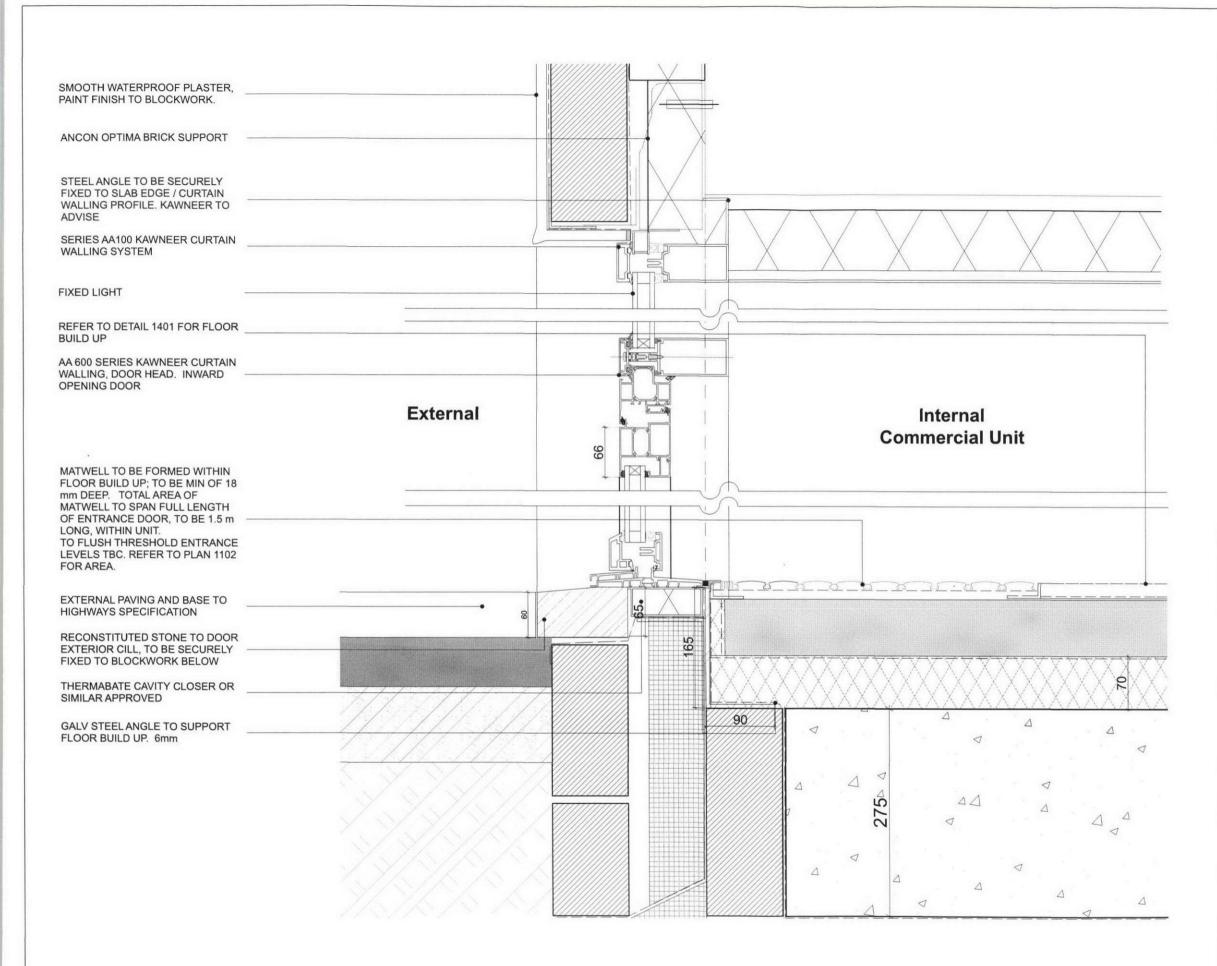
DETAIL 07 Section Retaining Wall / Door Threshold Commercial Unit
