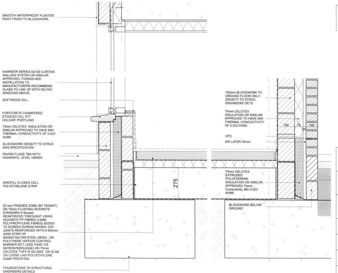
DETAIL 01 Section Retaining Wall
