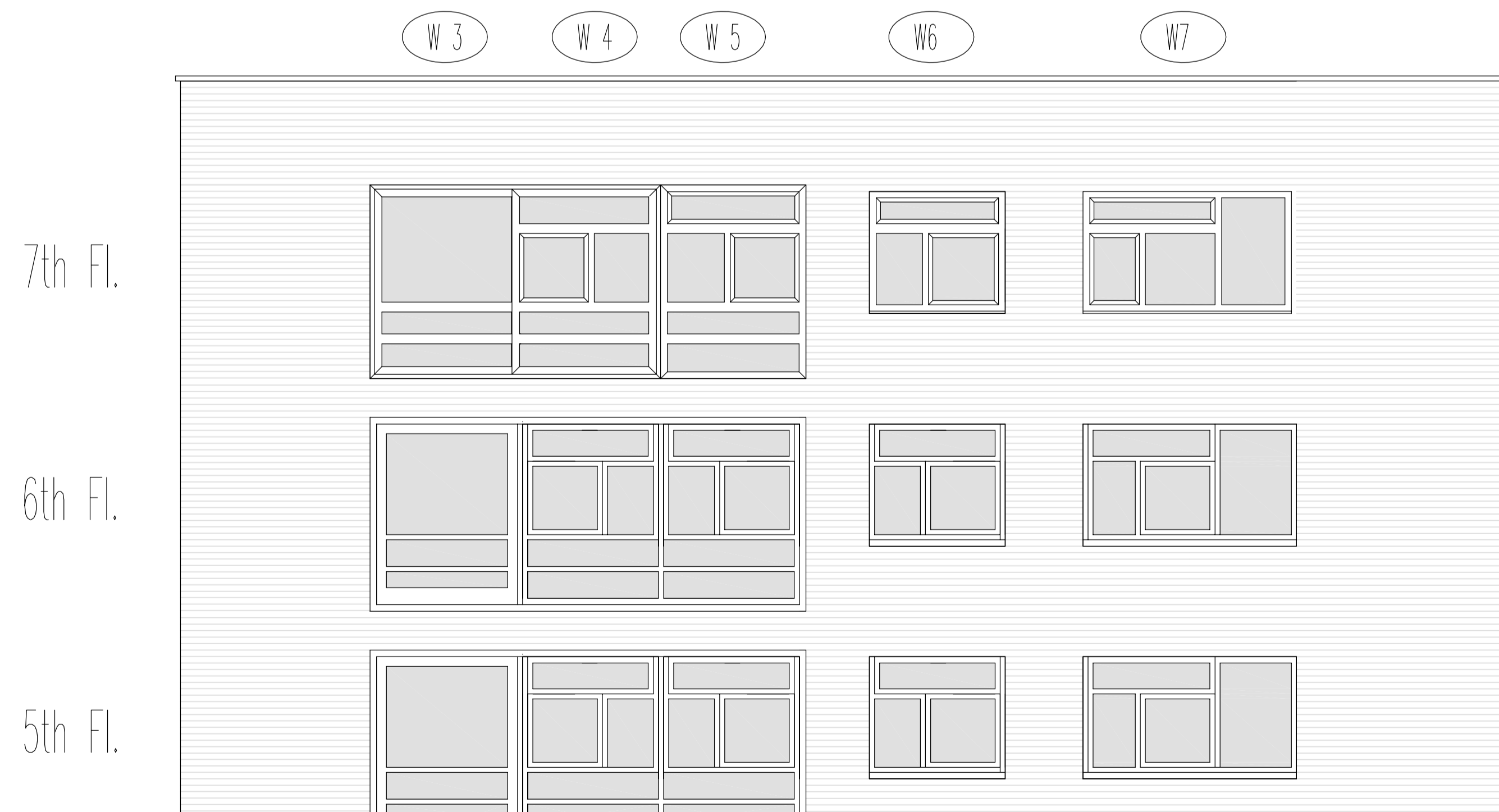
WEST ELEVATION (BALCONIES OMITTED) 7TH FLOOR AS PROPOSED, EXISTING AND APPROVED INDICATED ON LOWER FLOORS
