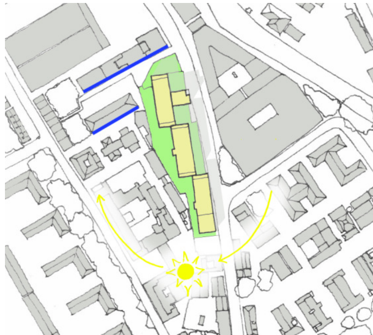
Fig - 6.5.2 - Sun Path Showing Shadows at Noon (Typical)
