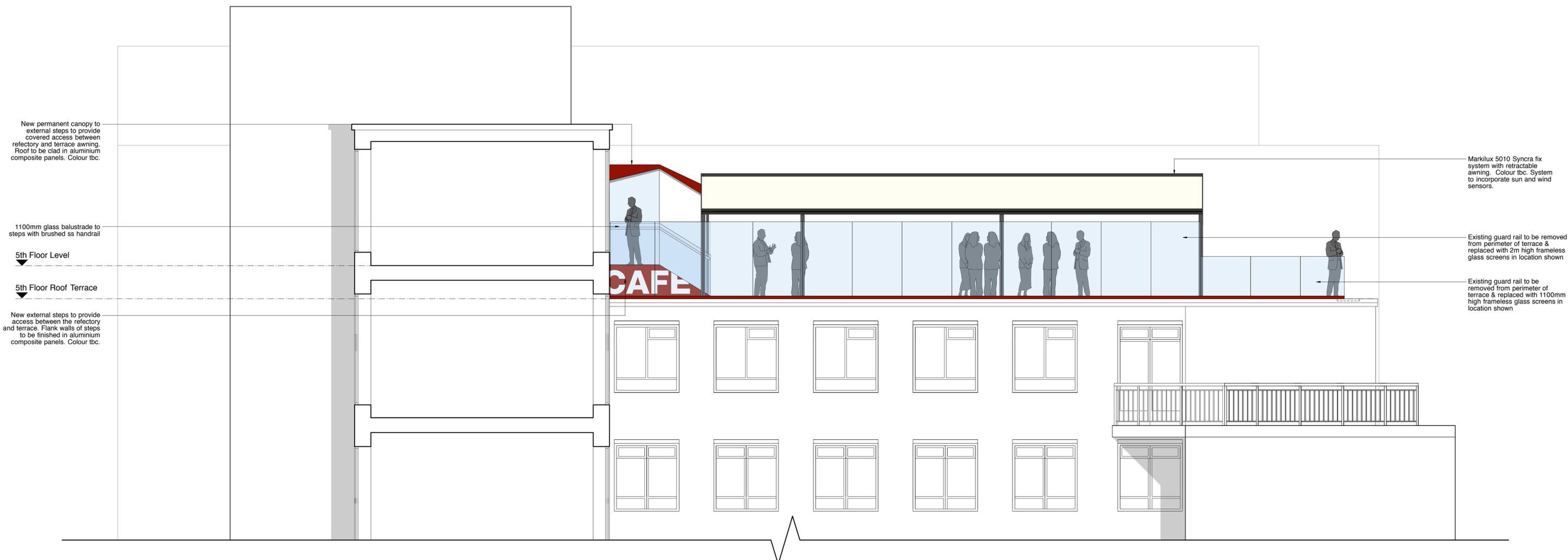
New permanent canopy to external steps to provide covered access between refectory and terrace awning. Roof to be clad in aluminium composite panels. Colour tbc.
