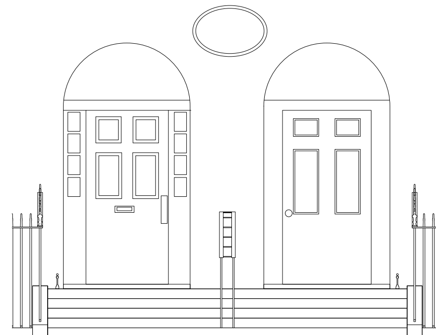
Entrance Elevation Scale 1:25
