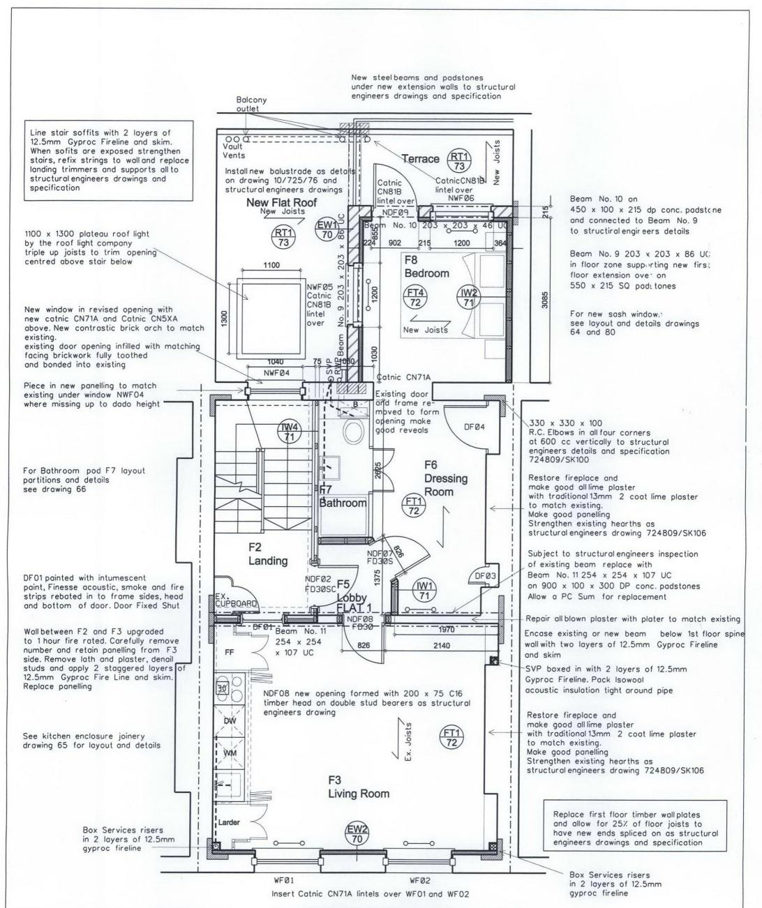
Ground, 1st, 2nd and 3rd floor joists strengthened at every third point of span with full depth noggins as structural engineers drawins 724809/BF/P1 and SK104 All non original glazing panes in WF01 and WF02 replaced with 4mm high performance acoustic glazing
