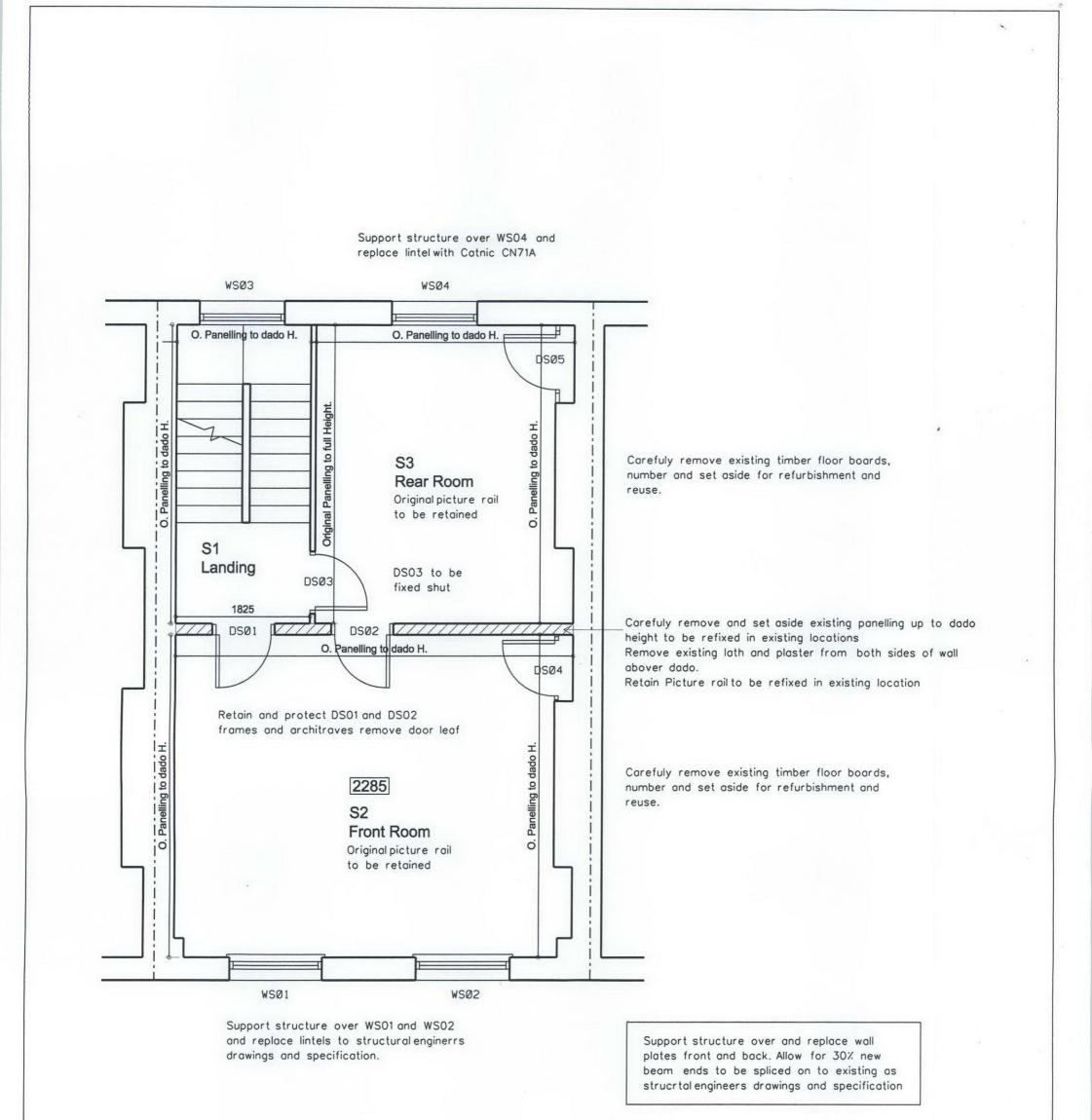
Carefully chase brickwork out at all four corners to allow for  $330 \times 100 \times 65$  RC concrete elbows 2 courses above floor and below ceiling and at 600 cc between all to structural engineers drawing 724809/SK100
