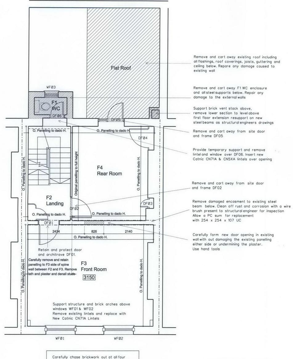
Carefully chase brickwork out at all four corners to allow for 330 x 100 x 65 RC concrete elbows 2 courses above floor and below ceiling and at 600 cc between
