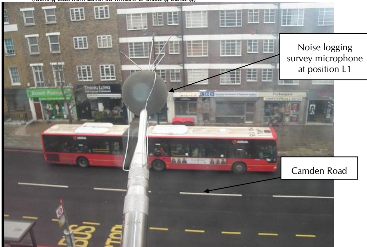
Figure A1 Measurement position L1 for PPG24 noise level logging (looking east from Level 03 window of existing building)
