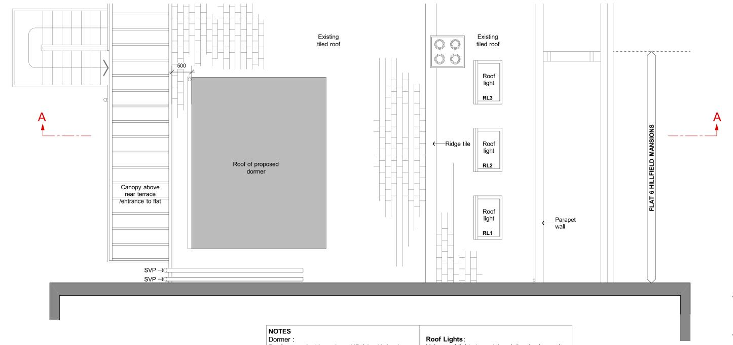
Roof covered with torch on HP felt with lead flashings and black UPVC gutter and rainwater downpipe.
