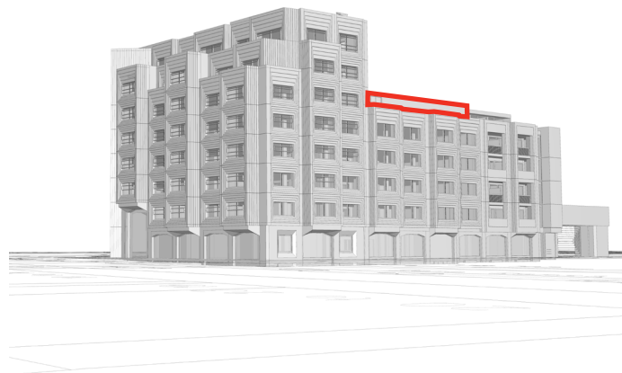
Iteration 02: plant consolidated and split into smaller enclosures arranged around the building and integrated into the tiered massing approach
