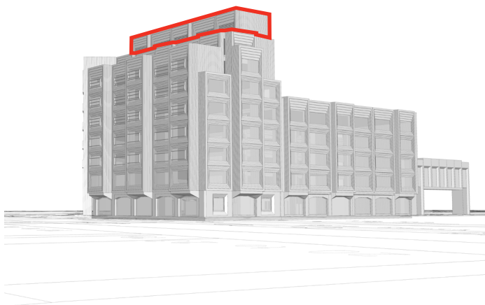
Iteration 01: plant consolidated and located in one enclosure fronting High Holborn
