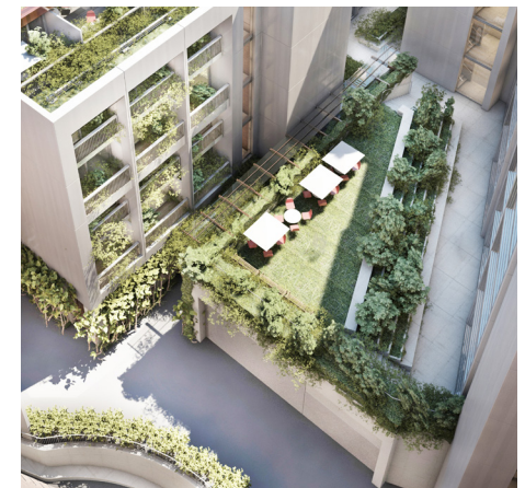
3 Service yard option 03: lower and upper garden providing at-grade garden access (first floor) and the head height required for vehicles
