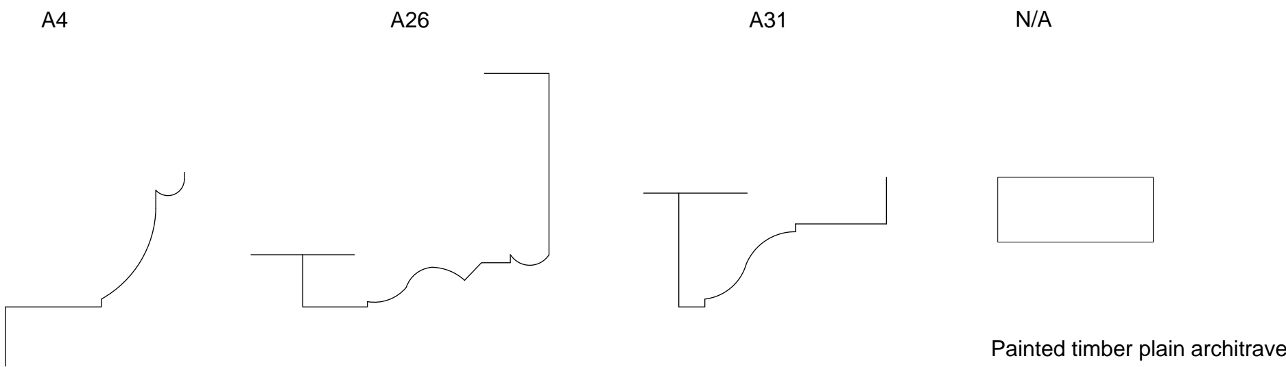
04 DOOR ARCHITRAVE TYPES A0425 EXISTING 1:2@A1
