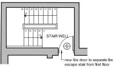
PROPOSED FIRST FLOOR PLAN HALF LANDING FIRE ESCAPE STAIR
