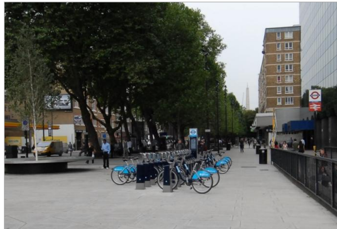
Figure 3.1: Double row docking station on footway
