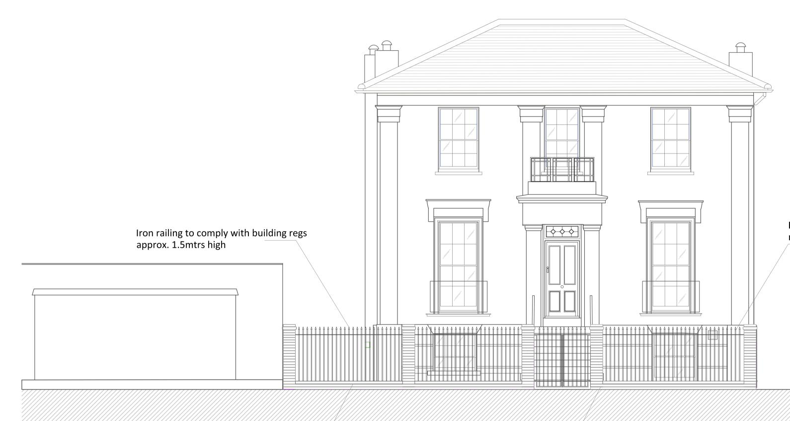
Final wall and railing height to match building render detail at indicated level
