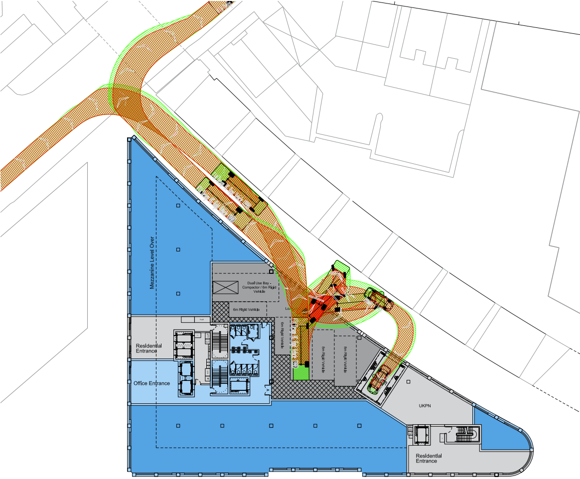
Swept path diagram showing vehicular movements at the loading bay and car lift
