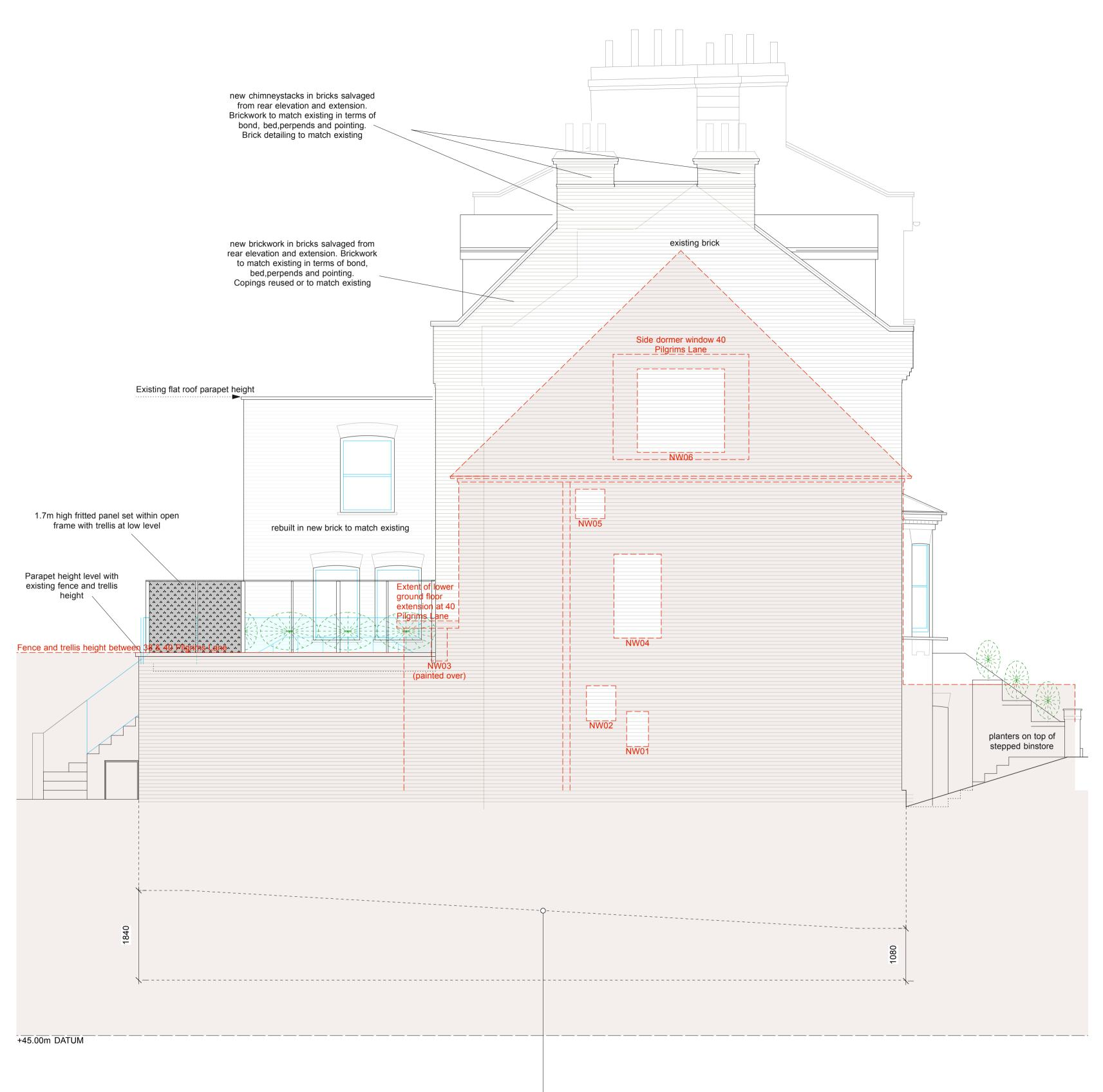
Likely depth of new foundations & under-pinning required if the basement is not constructed.
