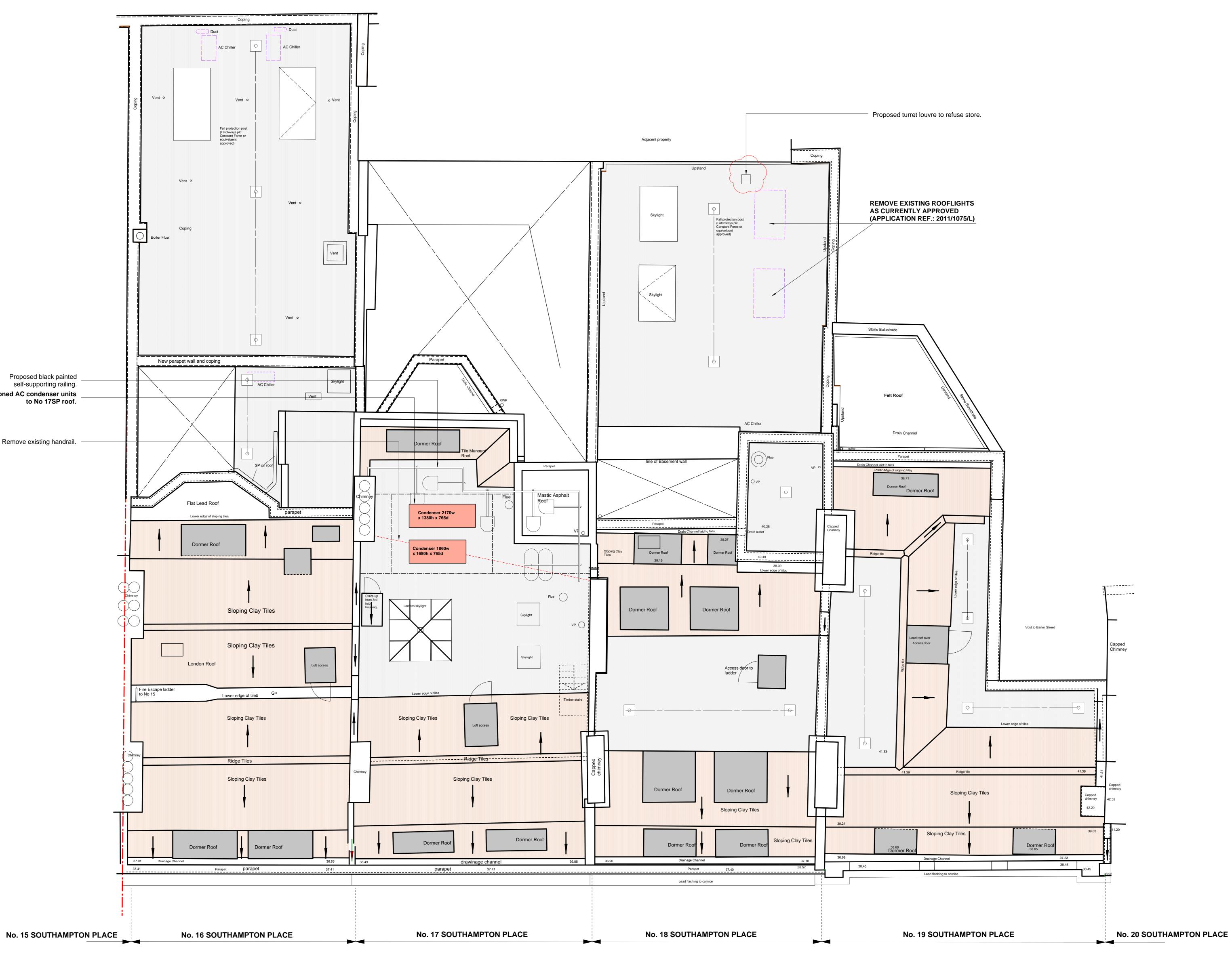
Proposed black painted self-supporting railing. Repositioned AC condenser units to No 17SP roof.
